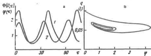
Fig. 1. a) Time dependence of gas temperature at the beam axis derived from the exact system (curve 1) and the approximate one (curve 2); b) phase pattern for approximate system (8) for the case of Fig. 1a. Parameter values  $\nu=3$ ;  $b=1$ ;  $j=2.905$ ;  $n_0=0.1$ ;  $\gamma=4.95$ ;  $R/x_0=5$ .
