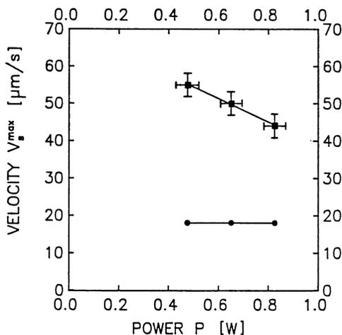
Figure 9. Scanning velocity  $v_s^{\max}$  referring to the maximum width of stripes achieved in laser direct writing of W lines from  $\text{WCl}_6 + \text{H}_2$ . The pressure was  $p(\text{H}_2) = 50$  mbar and ●  $p(\text{WCl}_6) = 0.49$  mbar, ■  $p(\text{WCl}_6) = 1.1$  mbar (Reproduced with permission from reference 8. Copyright 1993 Elsevier Science Publishers B.V.).
