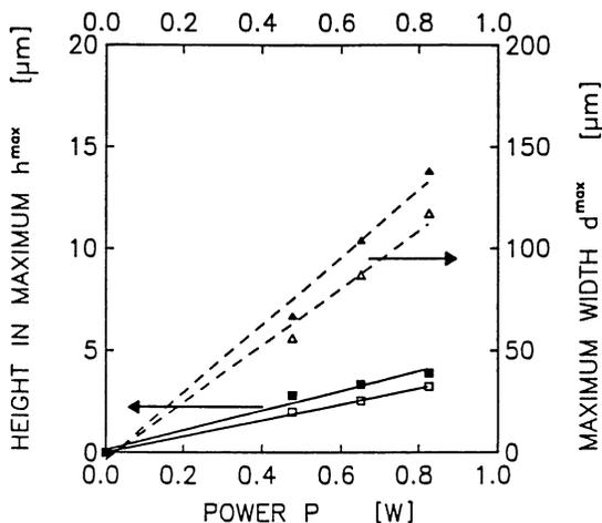
Figure 10. Maximum width and height of W stripes produced by laser direct writing from  $\text{WCl}_6 + \text{H}_2$ . The  $\text{H}_2$  pressure was  $p(\text{H}_2) = 50$  mbar. ■, ▲  $p(\text{WCl}_2) = 0.49$  mbar ; □, Δ  $p(\text{WCl}_2) = 1.1$  mbar (Reproduced with permission from reference 8. Copyright 1993 Elsevier Science Publishers B.V.).
