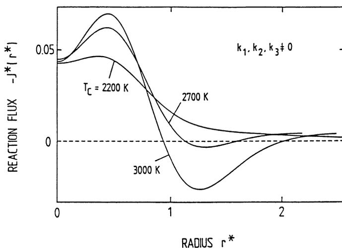
Figure 4. The normalized reaction flux as a function of  $r^*$  with  $k_1 \neq 0$ ,  $k_2 \neq 0$ ,  $k_3 \neq 0$ ,  $\Delta E_1/k_B = 15000$  K,  $\Delta E_2/k_B = 8000$  K,  $\Delta E_3/k_B = 10000$  K. The different curves refer to  $T_c = 2200$  K, 2700 K, 3000 K (Reproduced with permission from reference 6. Copyright 1992 Elsevier Sequoia).
