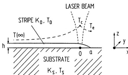
Figure 6. Schematic for direct writing. The coordinate system is fixed with the laser beam. The center of the laser beam with radius  $w$  is at the origin  $x = 0$ ; the forward edge of the stripe is at  $x = a$ .  $T_c$  and  $T_e$  are the corresponding temperatures. The temperature profile is indicated by the dashed curve. The height of the stripe is  $h$  and its width is  $d = 2r_D$  (Reproduced with permission from reference 8. Copyright 1993 Elsevier Science Publishers B.V.).
