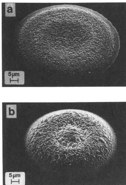
Figure 5. SEM pictures of W spots deposited from 0.49 mbar  $\text{WCl}_6$  + 400 mbar  $\text{H}_2$  by means of 680 nm dye-laser radiation a)  $P = 300$  mW,  $\tau_\ell = 20$  s b)  $P = 240$  mW,  $\tau_\ell = 40$  s (Reproduced with permission from reference 7. Copyright 1992 Elsevier Sequoia).
