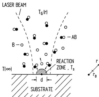
Figure 2. Schematic for laser-induced pyrolytic processing. The reaction zone is represented by a hemisphere of radius  $r_D = d/2$  whose surface temperature,  $T_S$ , is uniform. The gas-phase temperature is  $T_G(r)$ . The origin of the radius vector  $r$  is in the center of the hemisphere. The laser radiation is exclusively absorbed on the surface  $r = r_D$ . Carrier gas molecules, being possibly present, are not indicated.
