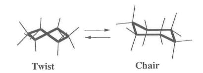
Fig. 3. The small carbon ring molecule cyclohexane can exist in different conformational states. The most stable forms are the twist and chair. The energy from thermal fluctuations causes the molecule to spontaneously switch between these conformational states.
