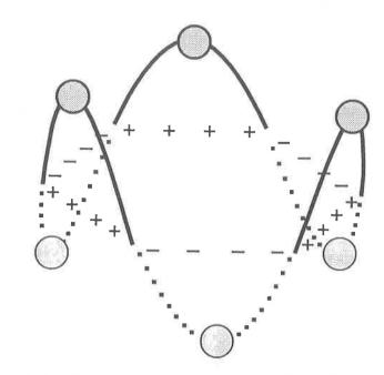
Fig. 5. The method used to encode the spatial structure of cyclohexane in the values of the nodes of the Hopfield network. The nodes of the network correspond to spatial positions around the carbon ring. If the atoms or the bonds connecting them are below the plane, the value of the corresponding node is -1. If the atoms or the bonds connecting them are above the plane, the value of the corresponding node is +1. The values of -1 and +1 are represented here as - and +.
