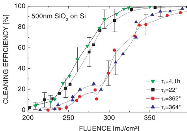
**FIGURE 4** Cleaning efficiency vs. storage time for 500-nm SiO<sub>2</sub> on (100) Si and 248-nm KrF laser radiation ( $\tau = 28$  ns). The pressure within the chamber was  $p < 2 \times 10^{-4}$  mbar after 3 h pumping and heating to 37.7 celsius
