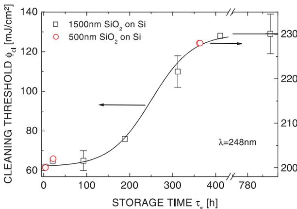
**FIGURE 2** Dependence of the cleaning threshold on storage time derived from the data in Figs. 1 and 4. The solid curve is calculated from (1)
