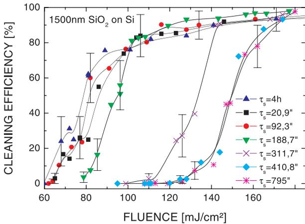
**FIGURE 1** Cleaning efficiency vs. storage time for 1500-nm  $\text{SiO}_2$  on (100) Si and 248-nm KrF laser radiation ( $\tau = 28 \text{ ns}$ ). The pressure within the chamber was  $p < 1.6 \times 10^{-4} \text{ mbar}$  after 3 h pumping and heating to  $37.9 \pm 0.3 \text{ celsius}$
