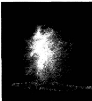
Figure 4: Plume expansion from a steel target
