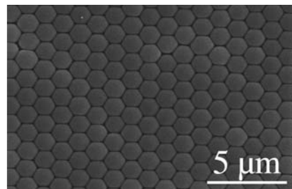
FIGURE 1 Scanning electron microscope (SEM) picture of a 2D lattice of quartz (a-SiO 2 ) microspheres of diameter d = 1.42 \mu\text{m} covered with a 125 nm layer of a-Si. The support is a 1.0 mm thick a-SiO 2 platelet
