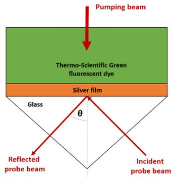
Fig. 2. Schematic of SPP excitation in the Kretschmann-Raether configuration.
