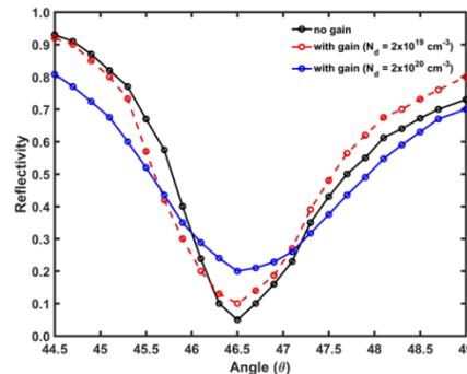
Fig. 3. Reflectivity with respect to incident angle ( $\theta$ ) with and without gain at different concentrations of dye molecules.
