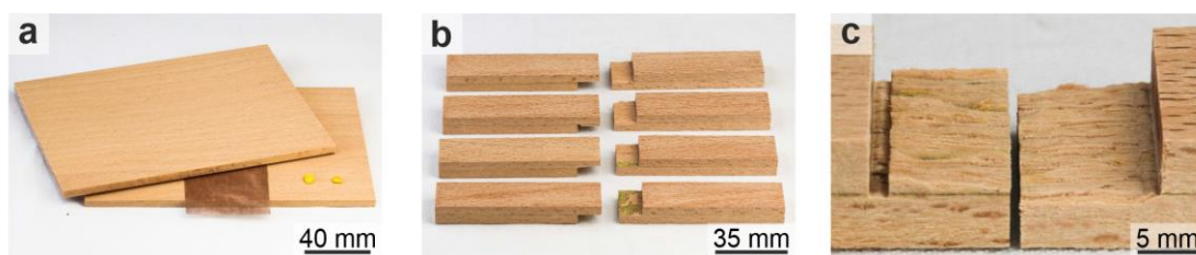
Figure S8. Preparation and results of the tensile shear test measurements. a) Two wooden plates with a size of 5 \times 125 \times 175 \text{ mm}^3 were glued together. The sensor was placed in between. b) Four samples were cut out from the glued plates and pulled apart until breakage. c) A sample with a WPF of 100%.
