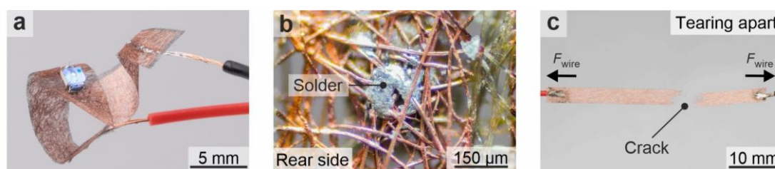
Figure S1. Solder joint on the porous and highly flexible paper substrate. a) Twisted electrode with the operational built-in activated LED visualizes the high strength of the solder connections. b) Rear side of a solder joint, which shows that the solder permeates through the metallized paper fibers. c) iSens paper substrates with soldered wires typically rupture in the bulk when the applied tensile force exceeds the intrinsic fracture strength of the substrate, while the solder joints on both ends remain intact.
